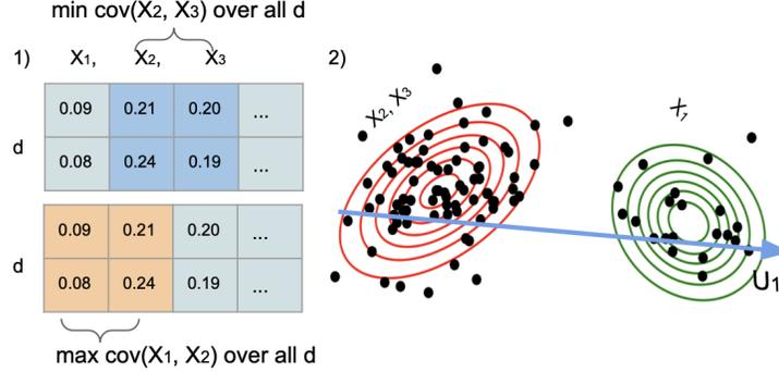
**Fig. 1.** The intuition behind PCA-BC: 1) Transpose  $X$  and visualise the nodes with the maximum and minimum covariance ( $\text{cov}(\cdot)$ ) in between; 2) Normalize transposed  $X$  and find the direction of maximum covariance by PCA.
